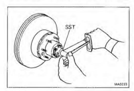
(e) Using SST, tighten the lock nut. SST 09607-60020
